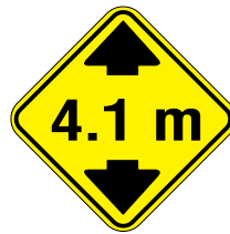
Low structure clearance 4.1 metres
