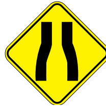
Pavement narrows ahead
