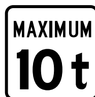
Weight restriction for a roadway or bridge of 10 tonnes
