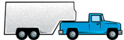
Truck pulling a trailer with a GVW of more than 4,540 kg (Class 3)
